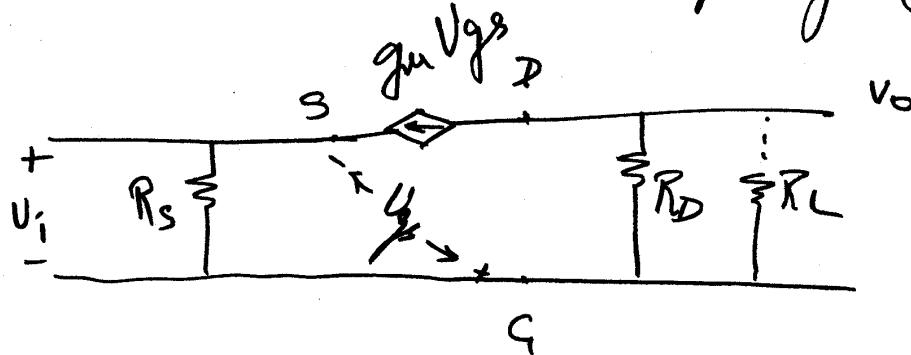
$$Z_i = R_s \parallel \frac{1}{g_m} \quad Z_o = R_D$$
